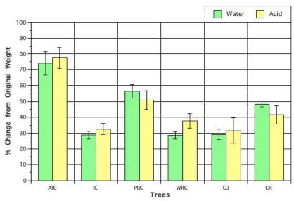
Figure 3. Water Absorption: Heartwood Samples in Water and Acidified Water  $N=4 \ Error \ bars = 1 SD$
