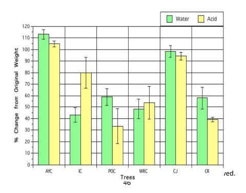
Figure 2. Water Absorption: Sapwood Samples in Water and Acified Water N=4 error bars = 1SD
