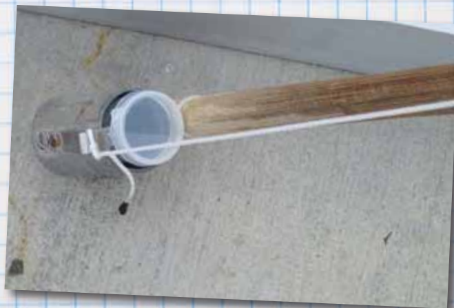
THE OPERATORS FOUND SUCCESS USING A DIPPER POLE ATTACHED TO A BACTERIOLOGICAL SAMPLE CONTAINER. BY OPENING THE HINGED LID AT A DESIRED DEPTH, THE WATER MIXED WITH THE DYE. THE OPERATORS ALSO USED THIS DEVICE TO COLLECT SAMPLES AT VARYING DEPTHS; THOSE SAMPLES WERE TESTED FOR CHLORINE RESIDUAL TO CONFIRM MORE FORMALLY THE MIXING THAT THE DYE TESTS SHOWED.
