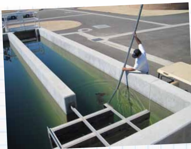
AN OPERATOR AT THE WESTERN MUNICIPAL WATER DISTRICT (RIVERSIDE, CALIF.) DELIVERS A DOSE OF DYE TO QUICKLY TEST HOW ADDING NEW BAFFLES AFFECTED THE CHLORINE CONTACT TANKS.
