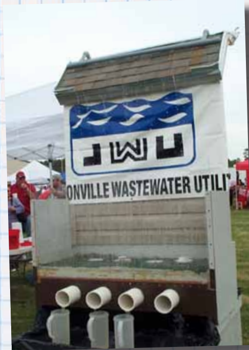
THE DISPLAY SIMULATES WHAT HAPPENS WHEN RAIN RUNS OFF OF ROOFS AND FALLS ONTO CLEAN-OUT CAPS. THE EXCESS INFILTRATION AND INFLOW LEADS TO STRESS ON THE DOWNSTREAM TREATMENT FACILITY.
