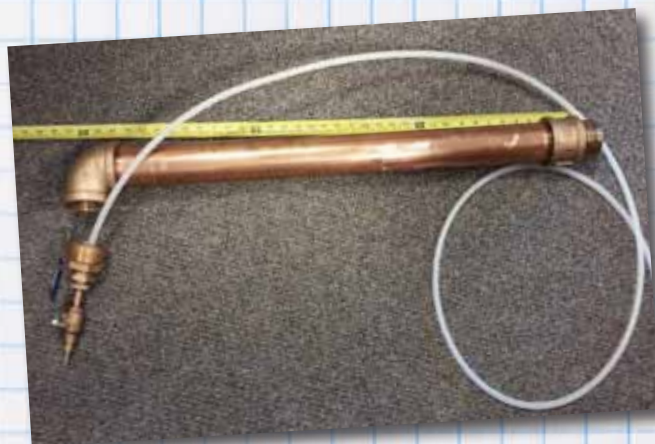
BY USING TUBING INSIDE BLOW PIPES, HRSD OPERATORS WERE ABLE TO REDUCE THE AMOUNT OF GAS TO BE PURGED FROM 3 L TO 0.3 L. THIS CHANGE HELPED TO COLLECT MORE RELIABLE HEADSPACE GAS SAMPLES.
