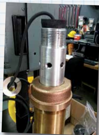
USING AN IN SITU OPTICAL DISSOLVED OXYGEN PROBE – SEEN HERE INSERTED INTO THE BOTTOM PORTION OF THE RISER PIPE – IN THE FORCE MAIN ELIMINATED WORRIES THAT PULLING SAMPLES OUT OF THE PIPE FOR MEASUREMENT WAS INTRODUCING EXTRA DISSOLVED OXYGEN.
