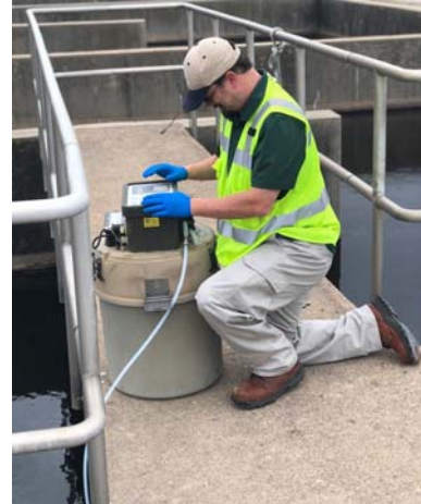
24-hour composite sampling event for source control program
