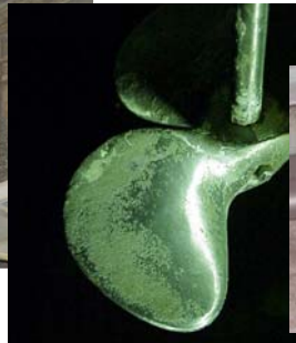
Deposits on mixer blade in dewatering centrate storage tanks
