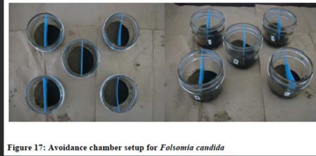
Figure 17: Avoidance chamber setup for Folsomia candida
