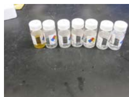
CHG aqueous feed (far left) and liquid effluent samples
