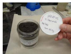
Solids from filter vessel
