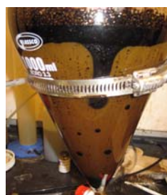
HTL steady state liquid effluent
