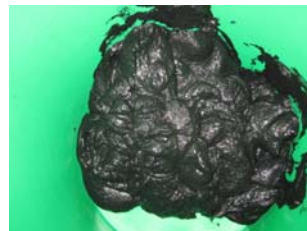
Post-digester (16.4 wt % solids)
