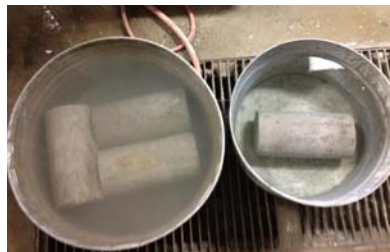
Concrete Coupons Curing
