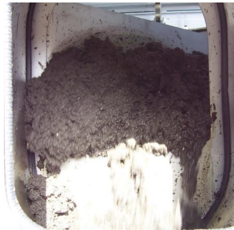
Figure 2. Photograph of typical thickened waste activated sludge.
