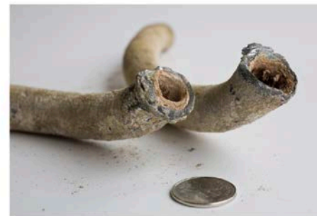
Lead pipes removed from the ground in Halifax last year. Photo: Zane Woodford
