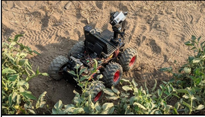
The "Spectra Rover" capturing RGB and IR images. (Photo credit: Pauline Estrada)
