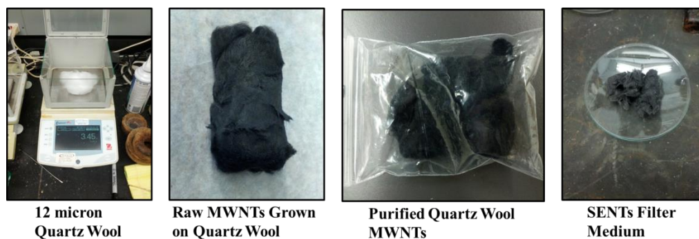
Figure 7. Progression of Filter Medium Preparation Stages
