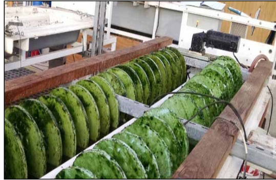
A Rotating Algal Biofilm Reactor (RABR) was used as a platform to grow microalgae on produced water
