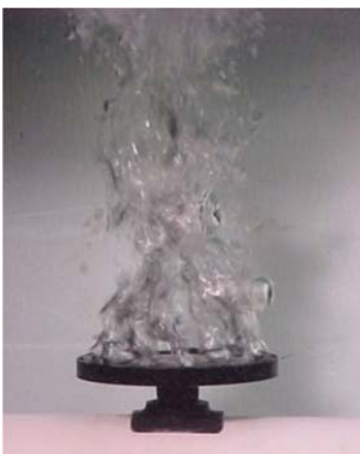
Figure 5. Coarse bubble diffuser 0.2 – 0.5in. in diameter [2]
