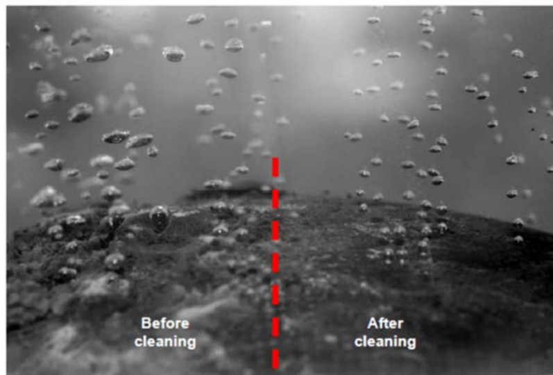
Figure 7—Aeration Bubble Size Before and After Cleaning. Photo courtesy of Dr. Diego Rosso.
