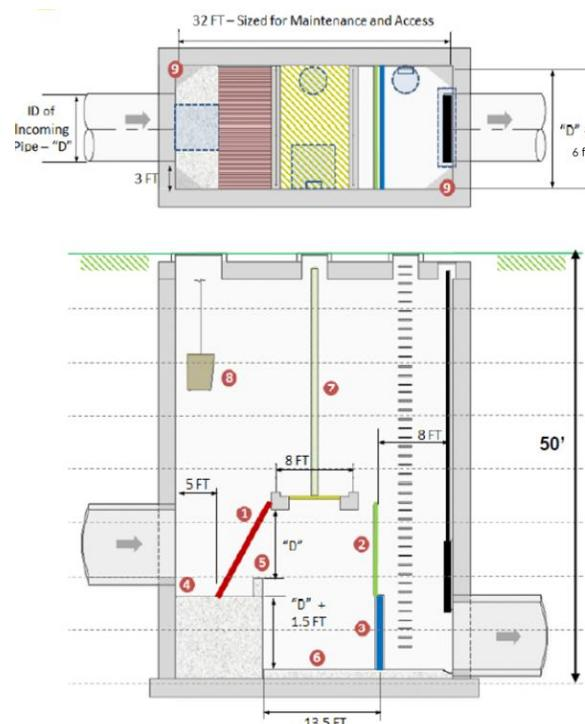
Figure 12 – Design for NEORSD's Near Surface Facilities which are installed at each drop gate along new tunnels.
