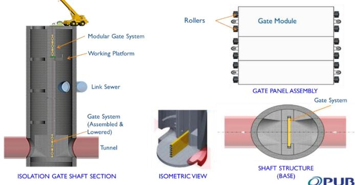
Figure 9 – Roller isolation gates concept developed by Singapore PUB.
