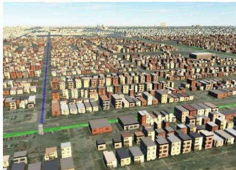
Figure 5 – 3D integrated layouts can show how the tunnels alignment will affect the community and other infrastructure. (Figure provided by: F. Oksuz)
