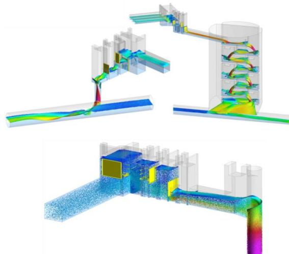
Figure 6 – An example of a CFD model for the different type of drop shaft connections. (Figure provided by F. Oksuz)
