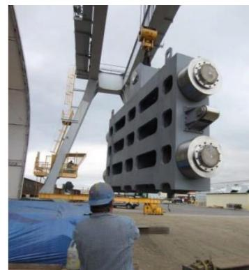
Figure 14 – High head wheel gates for tunnels. (Photo provided by F. Oksuz)
