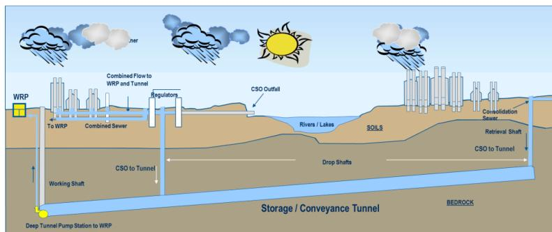
Figure 2 – An overview of deep tunnel systems for CSO control.
