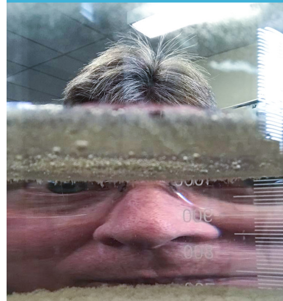
Mixed liquor sample from the aeration tank at the South Deerfield wastewater treatment plant showing smooth, compacted sludge with strong settling properties and crystal clear effluent.
